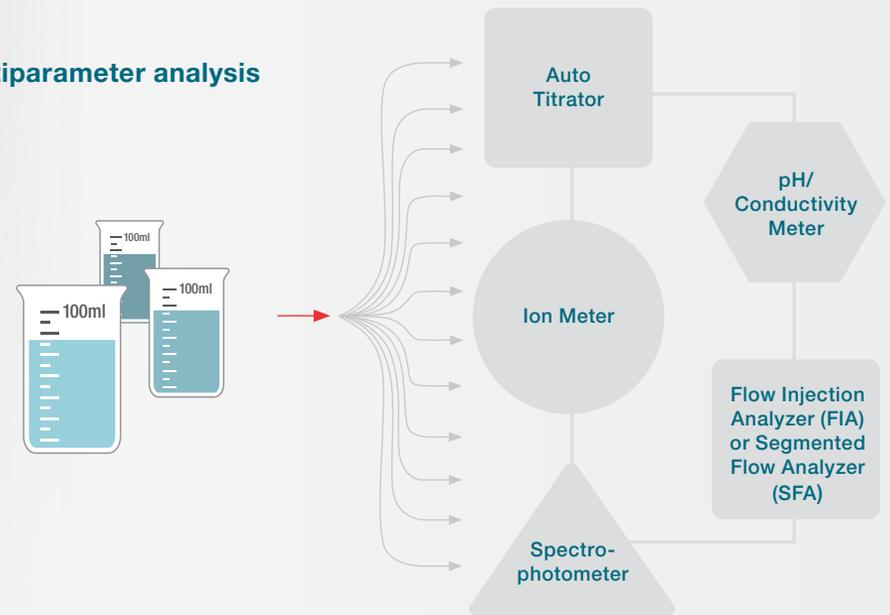
Traditional automated techniques, such as titration and continuous flow analysis, are relatively inflexible: dedicated modules are used for specific chemistries, and dedicated skilled technicians are needed for instrument operation and maintenance. Analyses are time consuming and generate a large volume of reagent waste.
