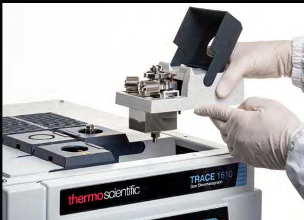
Access unprecedented flexibility. Switch instant-connect injectors and detectors in minutes without tools.
